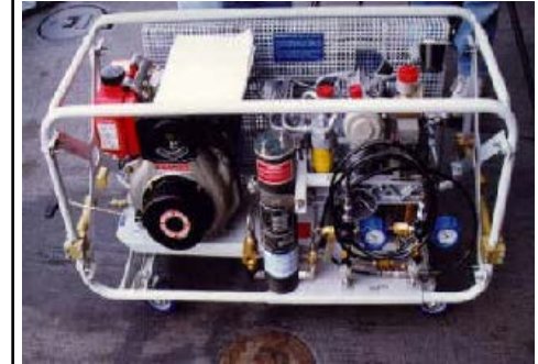
Diesel-Driven Air Compressor
