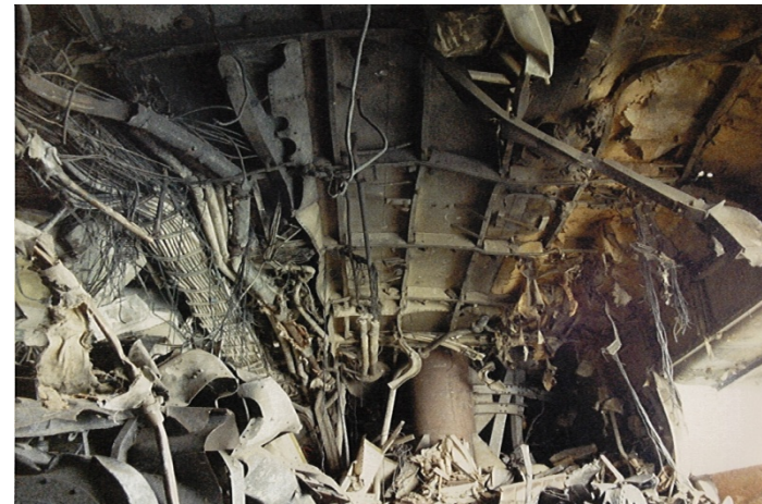
Several compartments in immediate area of impact demolished including IC shop and Operations berthing
