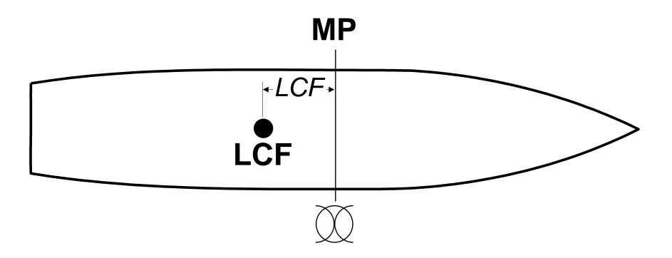
LCF - The Longitudinal Center of Flotation
