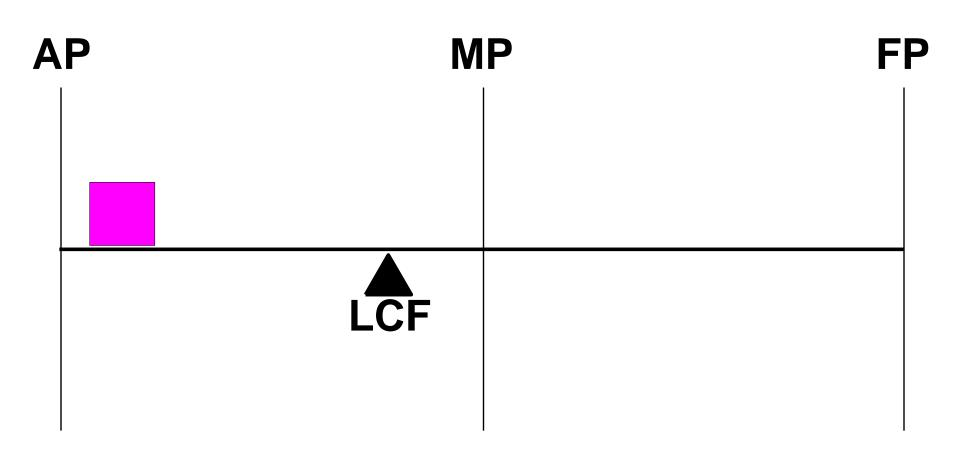
For a weight addition the Trimming Arm (TA) is equal to the distance from LCF to the center of the weight
