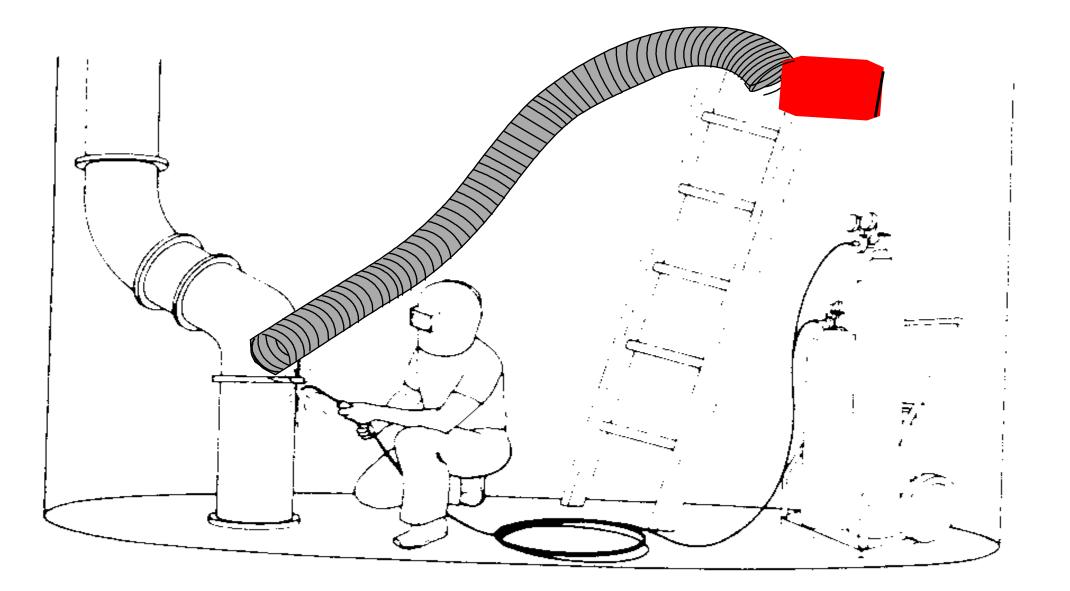
WARNING: ALWAYS SUPPLY PERSONNEL WITH NIOSH APPROVED RESPIRATORY PROTECTION EQUIPMENT FOR WORKING WITH HIGHLY TOXIC MATERIALS SINCE EVEN SLIGHT VENTILATION SYSTEM TROUBLE MAY RESULT IN SIGNIFICANT PERSONNEL EXPOSURE
