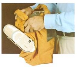
Hold the device by the open end of the hood with the life support pack away from the user.
