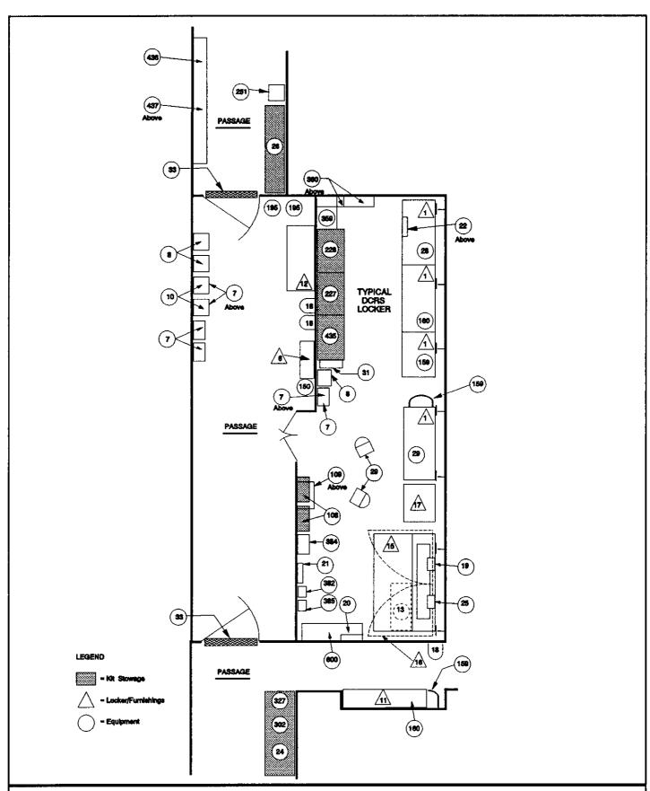
DAMAGE CONTROL EQUIPMENT STOWAGE SKETCH #002
